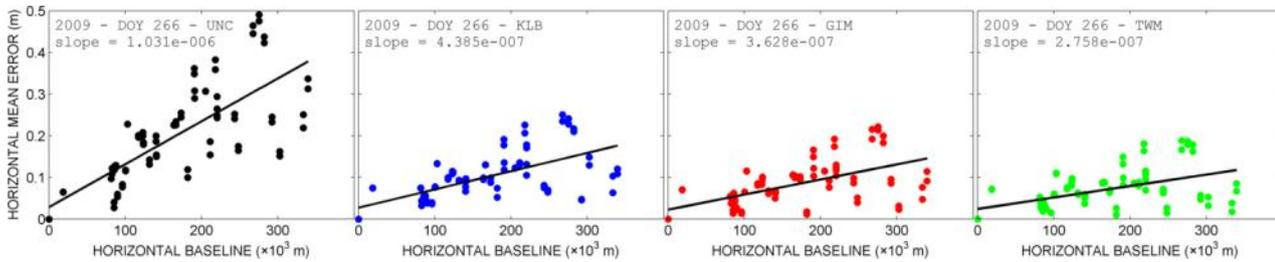
**Figure 2. Scatter plot of the horizontal mean error versus baseline vector without differential ionospheric correction UNC (col 1) and with differential ionospheric corrections using KLB (col 2), GIM (col 3), and TWIM (col 4) for DOY 266 of 2009 using differential positioning.**
