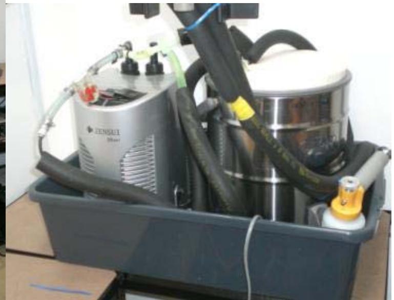
water circulator for FPI
