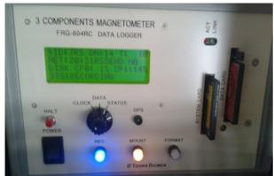
Figure 5: The 3-component magnetometer MAGDAS in Jerusalem, Ecuador.
