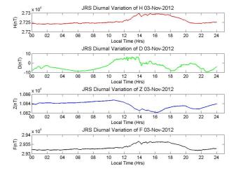
Figure 6: The daily variation of the magnetic field in the MAGDAS Jerusalem Station: H(horizontal component), Z(vertical component), D(deviation angle between H and X component) and F(the calculated geo-magnetic field)
