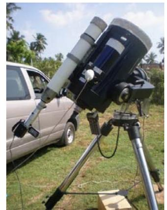
Fig. 1. Complete setup of the eclipse observation. 720 mm Vixen refractor and 1250 mm ETX Maksutov Cassegrain reflector were piggybacked on the 12 inch LX200 Mead with the tracking system.
