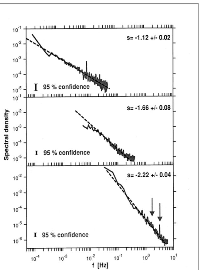
Fig. 6. Power spectra of solar wind ion flux variations for three ranges of frequencies [10]. The slopes of the spectra ( $s$ ) are written on the panels. Arrows mark the protons and alpha-particles' gyro-frequencies.
