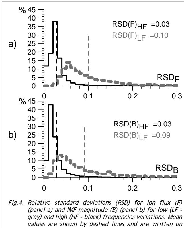
Fig.4. Relative standard deviations (RSD) for ion flux ( $F$ ) (panel a) and IMF magnitude ( $B$ ) (panel b) for low (LF - gray) and high (HF - black) frequencies variations. Mean values are shown by dashed lines and are written on the panels
