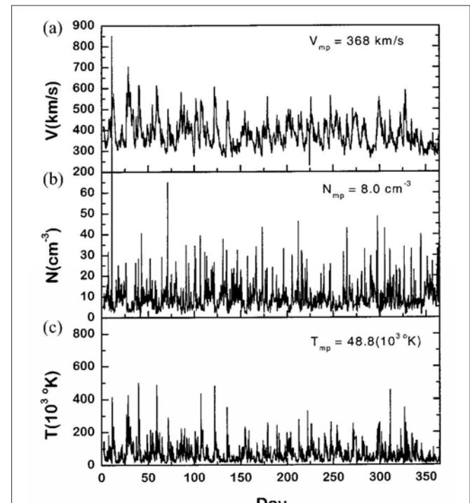
*Fig. 1. Variations of hourly-averaged values of solar wind velocity (a), density (b) and ion temperature (c) during 1997 by WIND data. Mean values are written on the panels.*
