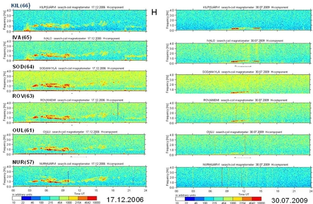
Fig. 1 The spectral structure of  $Pc1$  pulsations under magnetically disturbed period (left panel) and under very quiet conditions (right panel). The geomagnetic latitude of the stations is shown behind the station cod.
