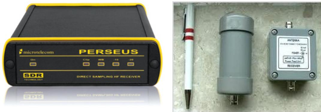
Fig. 3: Technical equipment of a GIFDS station: Perseus SDR receiver (left) and mini-whip antenna (right)
