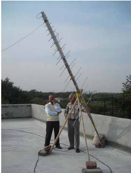
Fig. 1: Left: Subramaniam Ananthakrishnan (Pune) and Rajmal Jain (Ahmedabad) discussing the logarithmic-periodic antenna on top of the roof of the institute. It was manufactured by Somamshu Udyam out of standard aluminium profiles procured from a local store. The antenna is pointing to an average position of the sun transit. This (small) antenna covers 100 MHz – 1000 MHz. Another log-per covering 30 MHz -950 MHz is ready to be installed. The present design after Ashish Rojatkhar shows a very good reflection coefficient s_{11} over the whole band. The low noise 20 dB preamplifier is mounted on top of the antenna.
