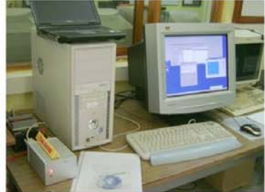
The CALLISTO Spectrometer is on the left side of the table (below 'TOBLERONE' chocolate) power supplies just behind the monitor with keyboard and PC on the right.
