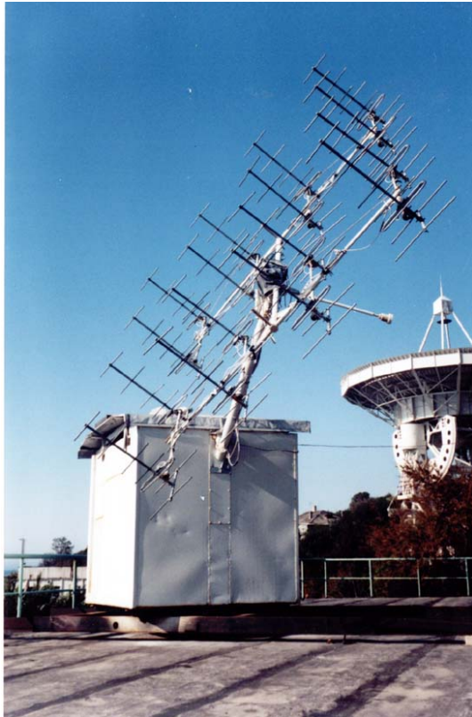
Fig. 2: Left: Phased array of 16 elements (4x4) with total size of 3.5x3.5 meter. Every element consists of 7 dipoles each. The frequency range is 250-350 MHz; the beam pattern is of order of 11°. The aerial is fixed on a parallactic mount with an electric drive to track the sun from 5 UT up to 13 UT. Preamplifier is a ZX60-33LN+ having a gain of 20 dB (placed in antenna box). Coaxial cable is 40 meters long with a loss of about 4 dB.
