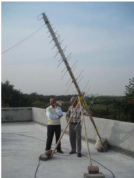
Fig. 1: Left: Subramaniam Ananthakrishnan (Pune) and Rajmal Jain (Ahmedabad) discussing the logarithmic-periodic antenna on top of the roof of the institute. It was manufactured by Somamshu Udyam out of standard aluminium profiles procured from a local store. The antenna is pointing to an average position of the sun transit. This (small) antenna covers 100 MHz – 1000 MHz. Another log-per covering 30 MHz -950 MHz is ready to be installed. The present design after Ashish Rojatkar shows a very good reflection coefficient s_{11} over the whole band. The low noise 20 dB preamplifier is mounted on top of the antenna.
