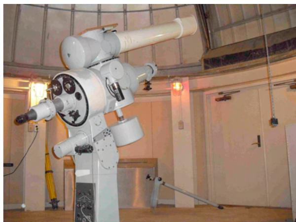
Figure 2 The 15 cm, F/15 Zeiss telescope (operational)
