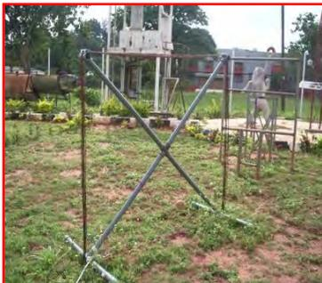
SID monitor VHF loop Antenna.
