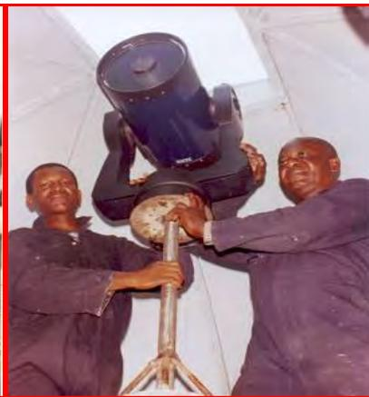
Optical Telescope Dome designed and constructed by CBSS Engineers with 25cm Meade LX200GPS OT inside the Dome.
