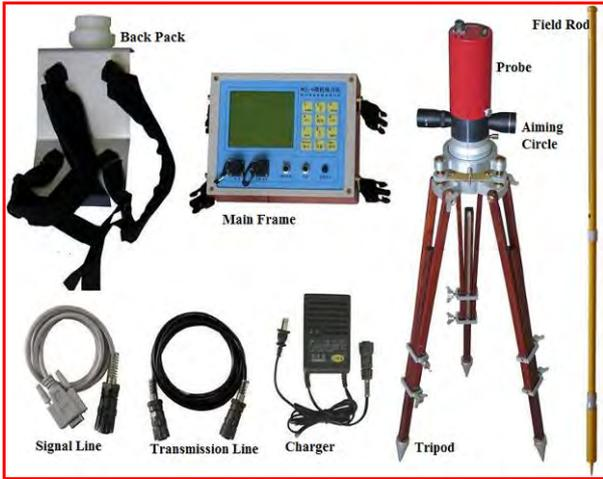
The Fluxgate Magnetometer.
