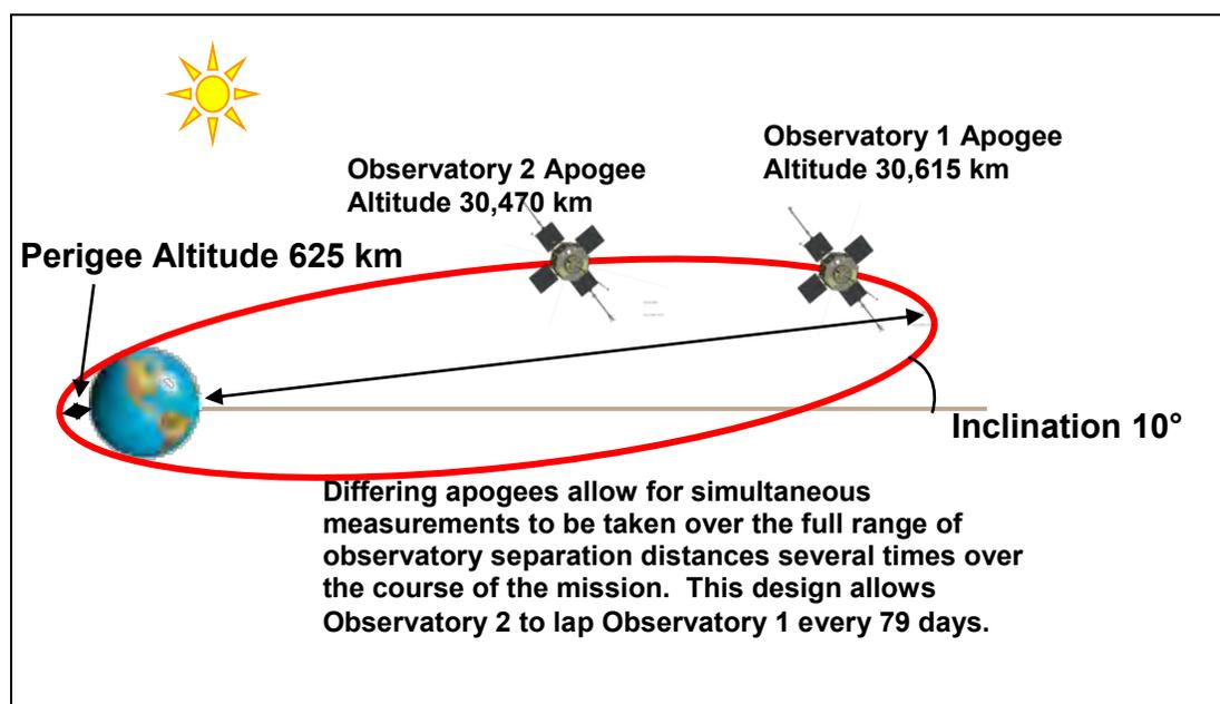
**Figure 1. Orbit configuration of the RBSP spacecraft**
