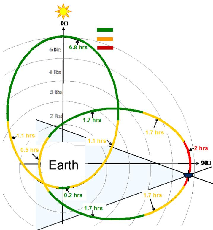
**Figure 4: Degree of antenna coverage due to seasonal variations**
