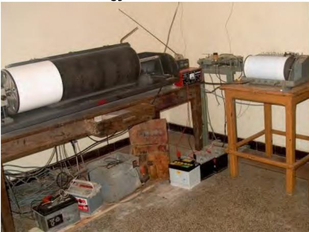
After the destructive earthquake of Agadir (1960) was the precursor of decision makers and therefore the need to create a seismic network has proven to be important and urgent. But it was only from 31 October 1964 that a three-component station coupled electromagnetic seismo-galvanized, short period, type APX, began recording at the observatory of Ifrane. The recordings were made on photographic paper.
