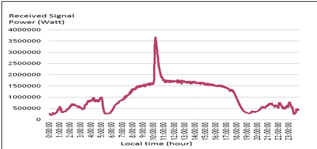
Figure 4. The spike showing the detected solar flare
