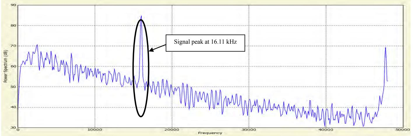
Figure 4. Clear peak at 16.11 kHz with amplitude 84.3 dB using SuperSID
