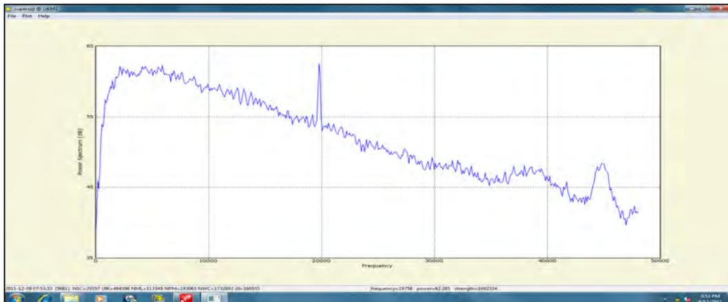
Figure 3. Receiving VLF signal from NWC station (freq: 19.8 kHz)
