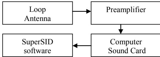
Figure 1. Block diagram of UKM-SuperSID
