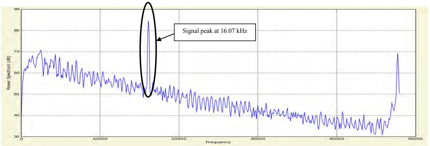
Figure 5. Clear peak at 16.07 kHz with amplitude 84.7 dB using UKM-SuperSID
