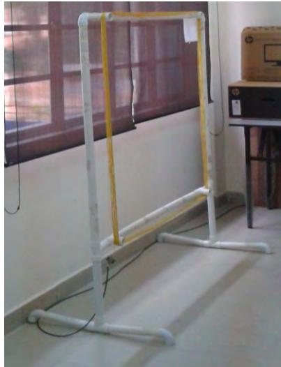
Figure 2. Loop antenna
