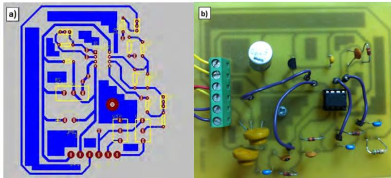
Figure 2. PCB layout a) before assembly and b) after assembled with components
