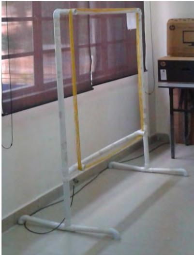
Figure 2. Loop antenna
