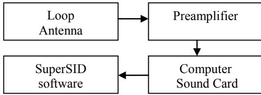
Figure 1. Block diagram of UKM-SuperSID
