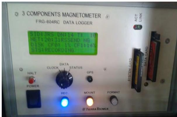
Figure 5: The 3-component magnetometer MAGDAS in Jerusalem, Ecuador.
