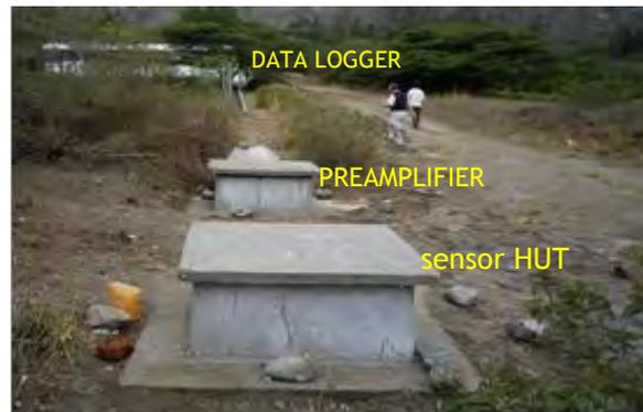
Figure 3: Houses for sensor HUT and preamplifier construction
