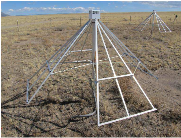
Long Wavelength Array (LWA) Cross-polarized, tied-fork dipole antenna 2-element, 10 ~ 90 MHz Ground mounted, mast included
