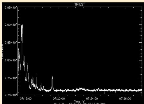
SRB detection pipeline: CALLISTO Spectrogram intensity plot
