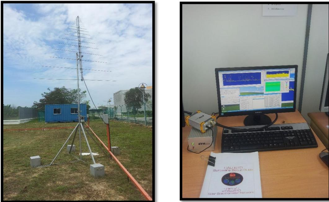
**Figure 1:** *The Log Periodic Dipole (LDPA) antenna and the CALLISTO spectrometer system at ANGKASA, Banting, Selangor, Malaysia.*
