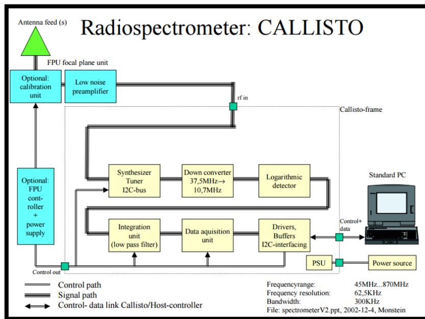
**Figure 3:** The configuration system of CALLISTO and LDPA at National Space Agency (ANGKASA), Banting, Selangor, Malaysia.
