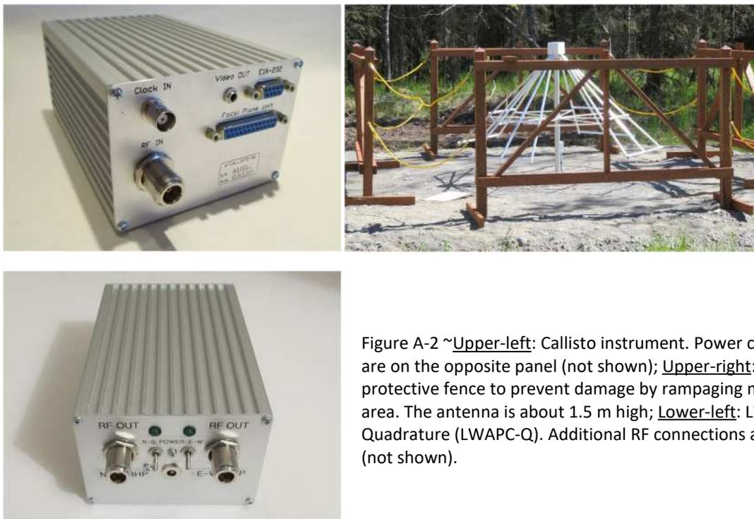
Figure A-2 ~Upper-left: Callisto instrument. Power connections and control are on the opposite panel (not shown); Upper-right: LWA Antenna with a protective fence to prevent damage by rampaging moose that frequent the area. The antenna is about 1.5 m high; Lower-left: LWA Power Coupler – Quadrature (LWAPC-Q). Additional RF connections are on the opposite panel (not shown).
