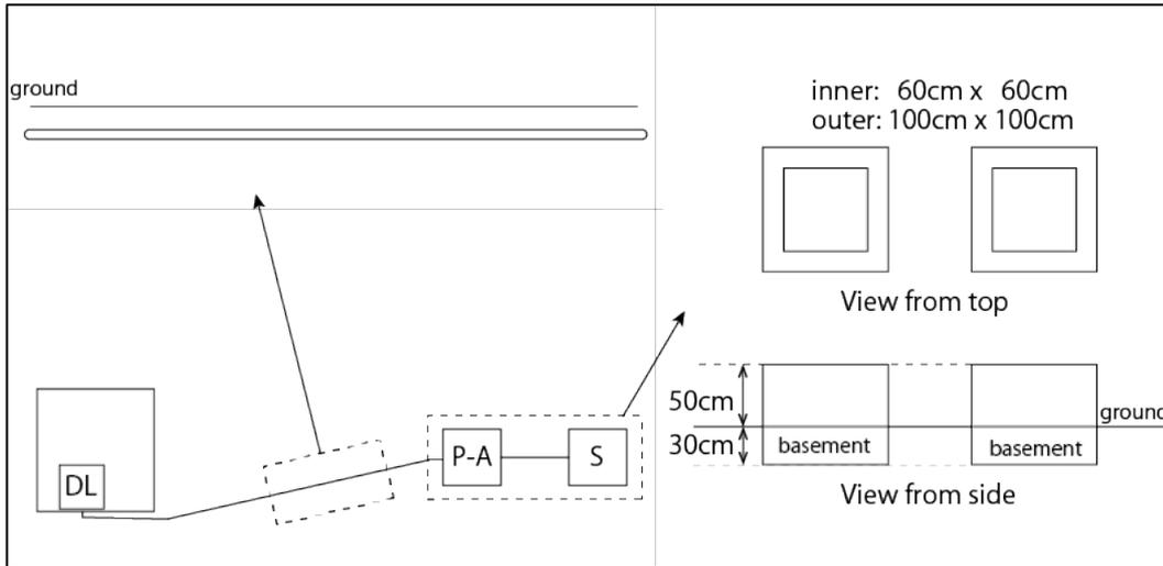
**Figure5. Design of MAGDAS instruments in TPT**
