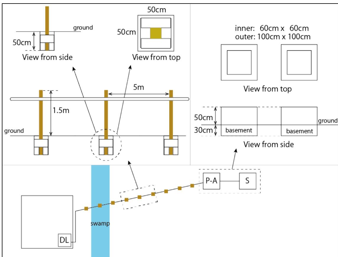
**Figure2. Design of MAGDAS instruments in TMA**
