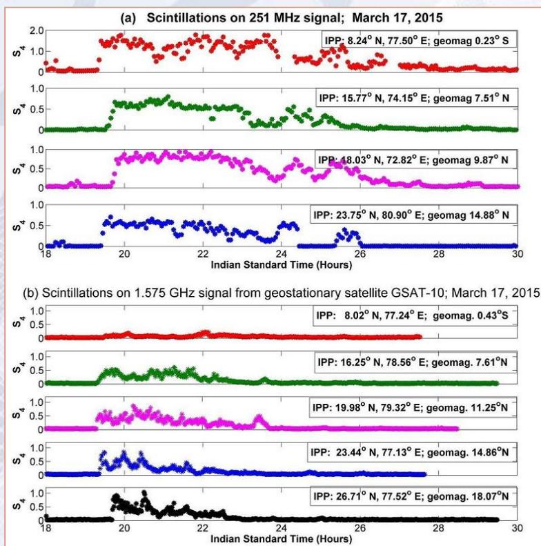
Variation of  $S_4$ -index with time for scintillations on (a) a 251 MHz signal transmitted from a geostationary satellite and recorded at four stations; (b) the 1.575 GHz signal transmitted from geostationary satellite GSAT-10 and recorded at five stations for which the signal path elevation angle was not less than 55°. Coordinates of ionospheric penetration points at 300 km are given.
