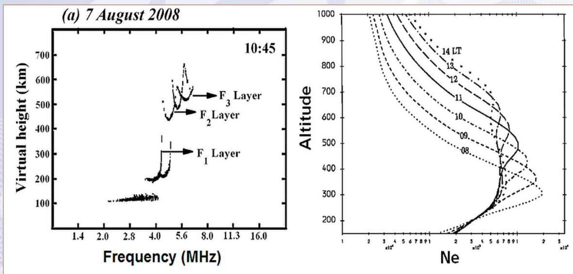
*The formation of F3 layer and modelled electron density profiles under the condition of strongest F3 layer from SUPIM model.*
