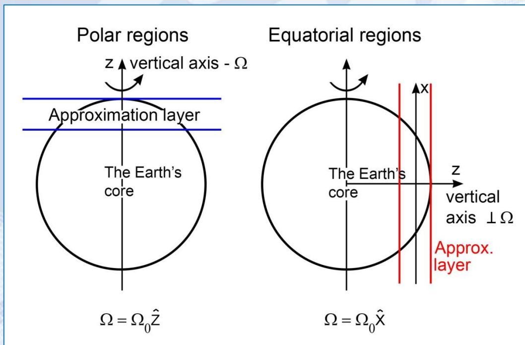
*Models of rotating magnetoconvection*
