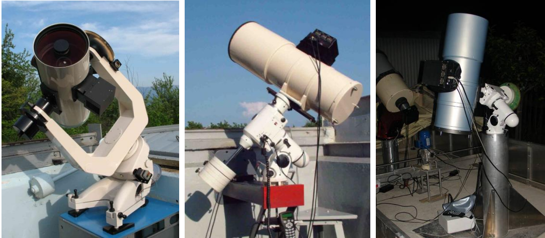
Fig. 6. 22 cm survey telescopes with FOV of 4°: PH-1 in Nauchny, ORI-22 in Ussuriysk, ORI-22 in Colleparado.
