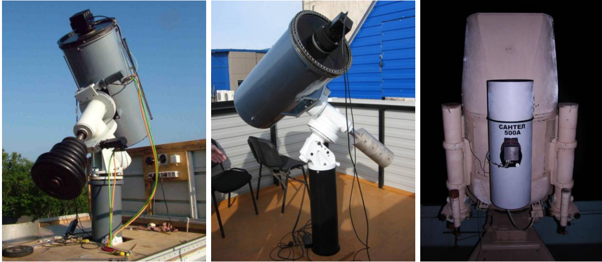
Fig. 8. New survey telescopes: 50 cm VT-50/400 (FOV is 1.8°) in Ussuriysk, 40 cm ORI-40 (FOV is 2.3°) in Krasnojarsk (second ORI-40 will be installed in Kitab in 2009) and 50 cm Santel-500a (FOV is 1.6° in Zvenigorod (over VAU camera mount).
