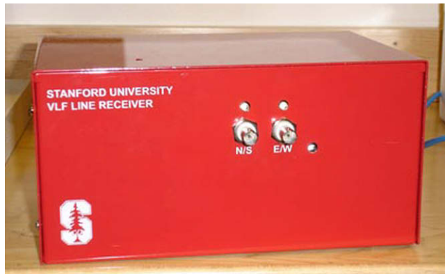
Fig. 1. AWESOME research-quality ionospheric monitor designed for universities.
