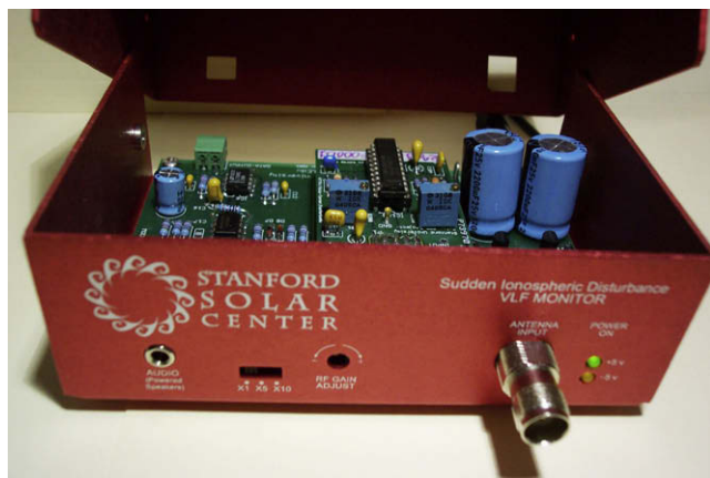
Fig. 2. SID ionospheric monitor, designed for high school use.
