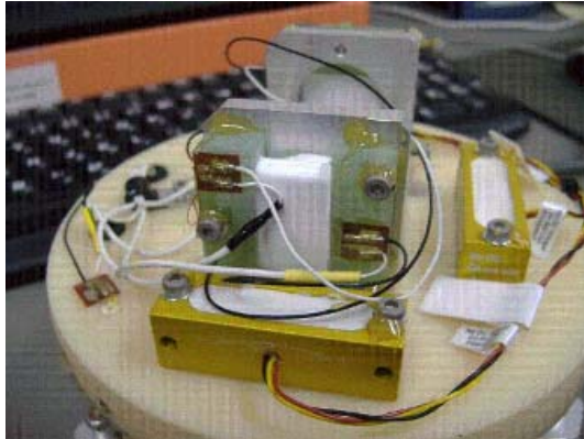
Fig. 3 This is the MAGDAS sensor with the round and black cover removed. The two brass-colored devices are precision tiltmeters. The rest form a tri-axial fluxgate magnetometer. This photo was taken at SERC by G. Maeda last year when the magnetometer had to be repaired (Colour online)
