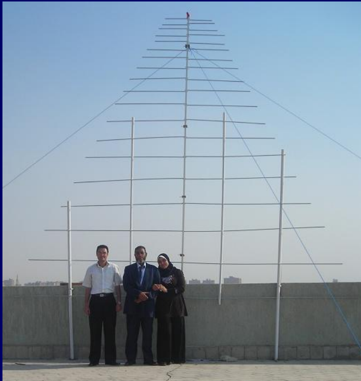
Left: Log-per 6m wide and 6m high 20 MHz – 175 MHz on the roof of SWMC. Right: 1st light two fast drifting type III bursts
