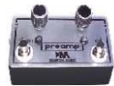
A PreAmp to raise very small signals to a level can be captured by a PC sound card.
