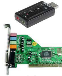
A sound card to convert signal from analog to digital.
