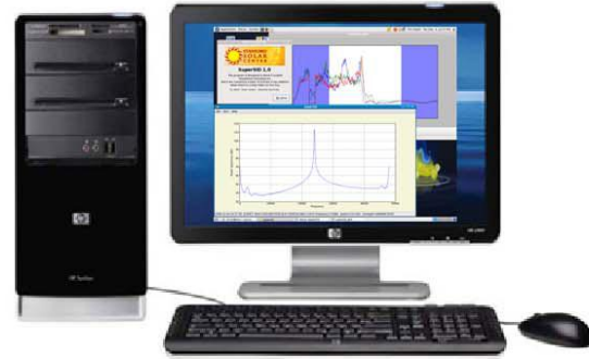
A PC to process data and estimate signal strengths through a day. Sudden Ionosphere Disturbance indicates Solar Flare on the SUN.
