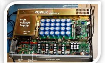
The 16-element main array (top left), the new fully digital radar hardware mounted in three racks (top right), one of the HF transceiver boxes (bottom left) and the internals of the power amplifier (bottom right) are located at SANAE IV in Antarctica
