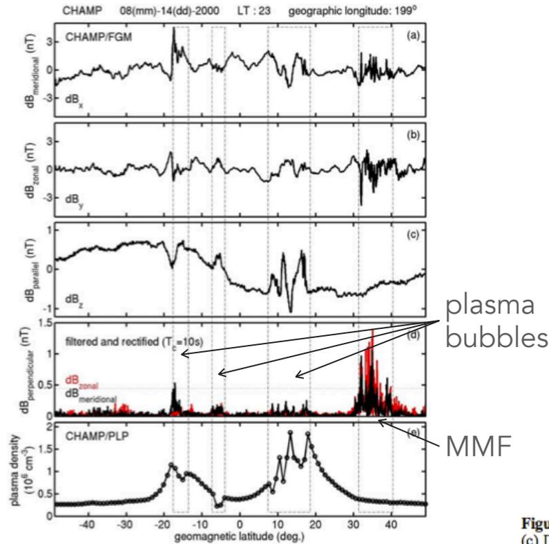
**Figure 1.** A typical example of midlatitude magnetic field fluctuation (MMF) at  $\sim 32^\circ$ – $42^\circ$  latitude. (a–c) Three respective components of residual magnetic field in mean-field-aligned coordinates. (d) Zonal and meridional components which have been high-pass filtered with a cutoff period of 10 s and then rectified. (e) Plasma density measured by CHAMP/PLP.
