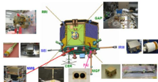
Figure 1. e-POP instrument payload layout on CASSIOPE.
