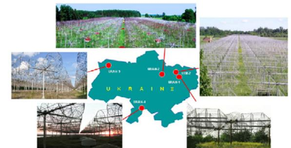
Figure 1. URAN decameter radio telescopes system on Ukraine map: Radio telescopes UTR-2 URAN-1, URAN-2, URAN-3 and URAN-4. They operate at the frequencies from 9 to 32 MHz.
