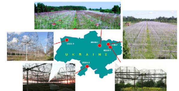
Figure 1. URAN decameter radio telescopes system on Ukraine map: Radio telescopes UTR-2 URAN-1, URAN-2, URAN-3 and URAN-4. They operate at the frequencies from 9 to 32 MHz.
