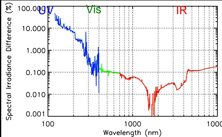
**Small variations in the visible (0.1%), but big changes in the UV. (UV, EUV and X-ray spectral irradiances are drivers of space weather)**
