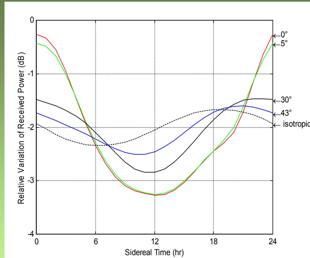
Received power at  $70^\circ\text{N}$  over a sidereal day for different antenna opening angles
