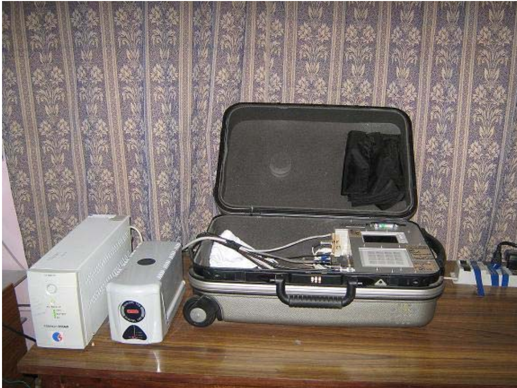
UPS, Isolation transformer and the Data logger
